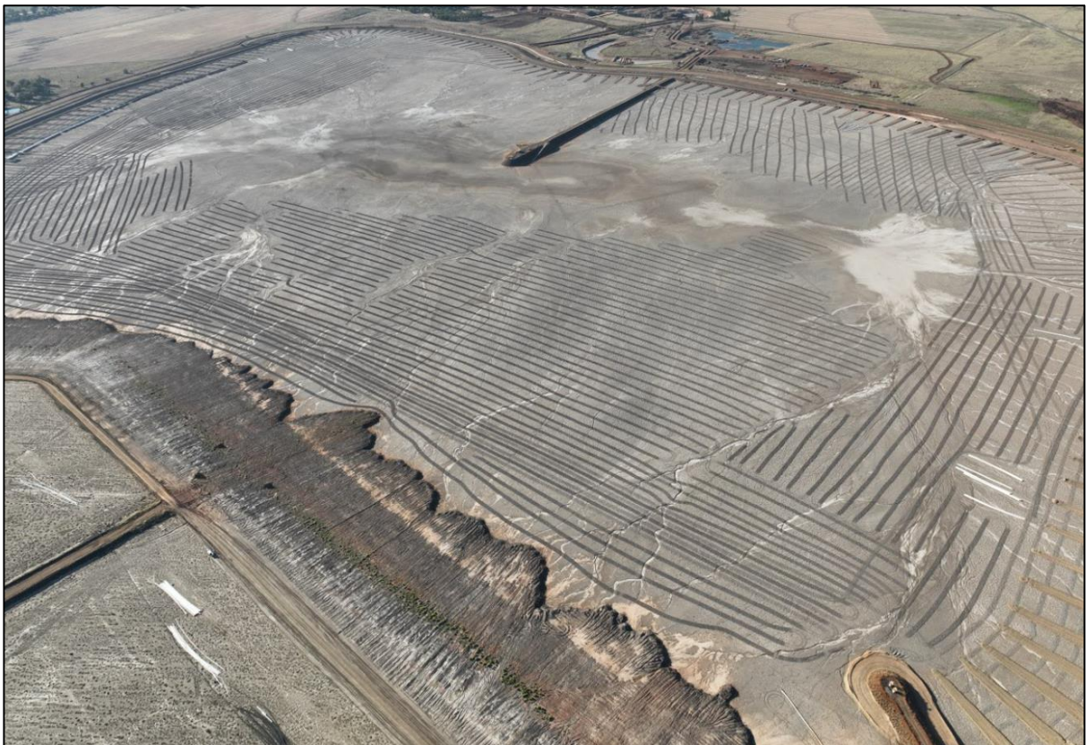
Figure 10 Ripping undertaken on Rosedale TSF for dust control
