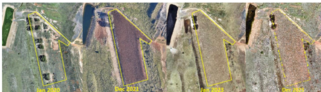
Figure 27 E22 waste rock batter rehabilitation repairs from 2020 to 2023
