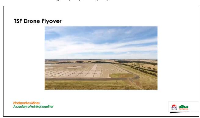
This short video shows an aerial view of our Tailings Storage Facilities, including our major dust mitigation measure – the crops growing on our TSFs. The advantage of this method is it gives us a greater understanding of the soil composition on our TSFs. We can also deposit tailings on top of the crops if need be. We are working on the closure of TSF1 in 2017.
